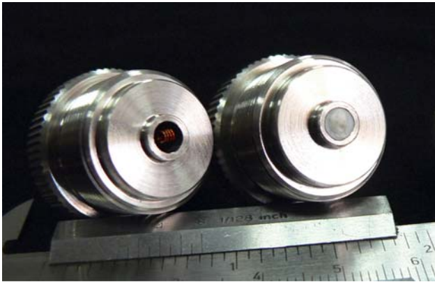
Fig. 1 Loop probe used for microwave measurements: before (left) and after filling the housing duct with epoxy resin to avoid perturbations to the acoustic field
